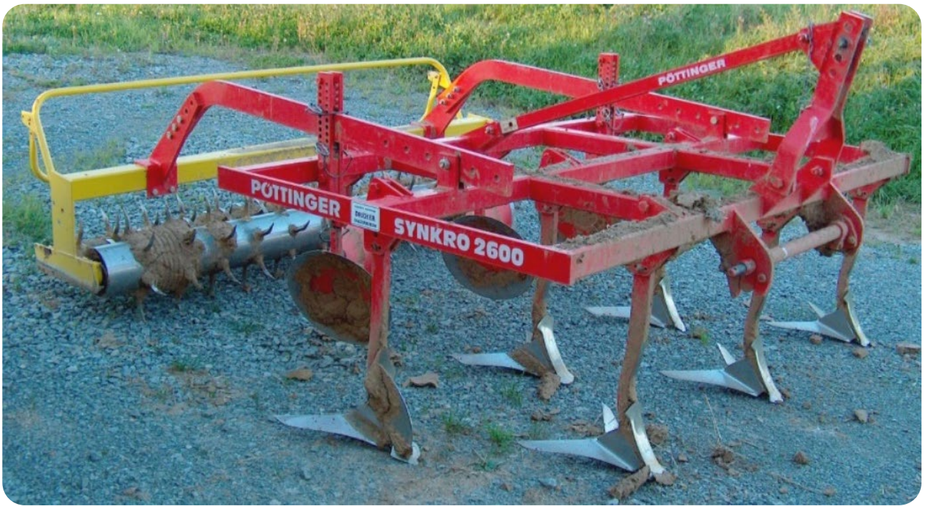
Figure 1. Wing share cultivator “Synkro 2600” by Pöttinger. Non inversion tillage does not mix soil layers keeping the original layering.
